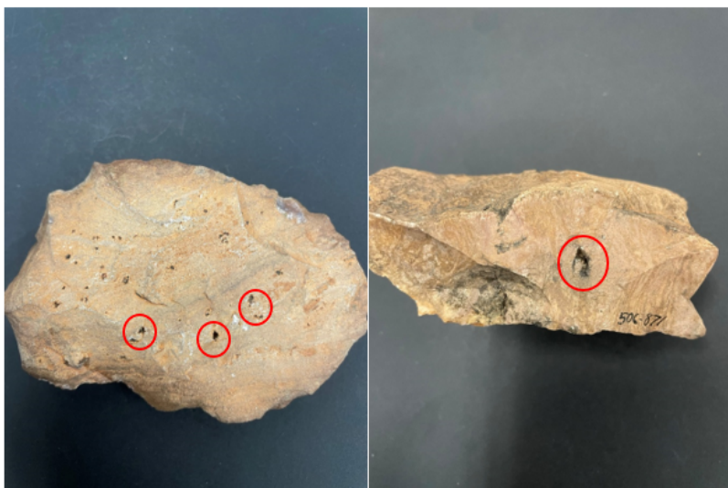
Figure 4.2.2. Examples of voids in Baker rhyolite (red circle indicates imperfection).
