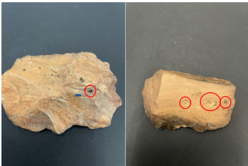
Figure 4.2.1. Examples of inclusions in Baker rhyolite (red circle indicates imperfection).
