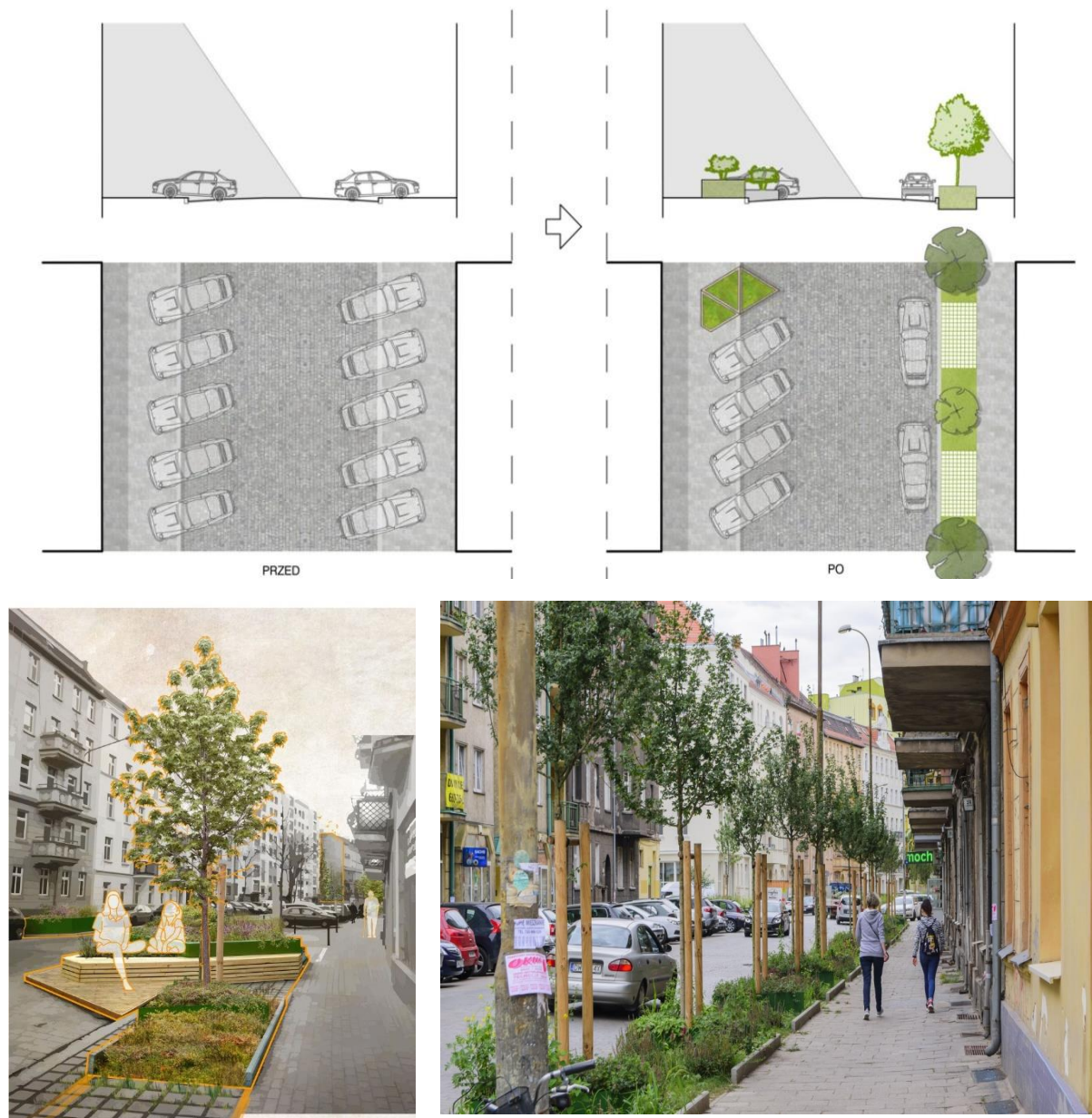
Fig. 39. Above - plan of the street fragment prior to its modification (on the left) and after the changes (on the right), at the bottom - a view of a place to sit under a tree and a row of trees along the pedestrian route; source: https://tecla.pl/portfolio/grow-green-2/
