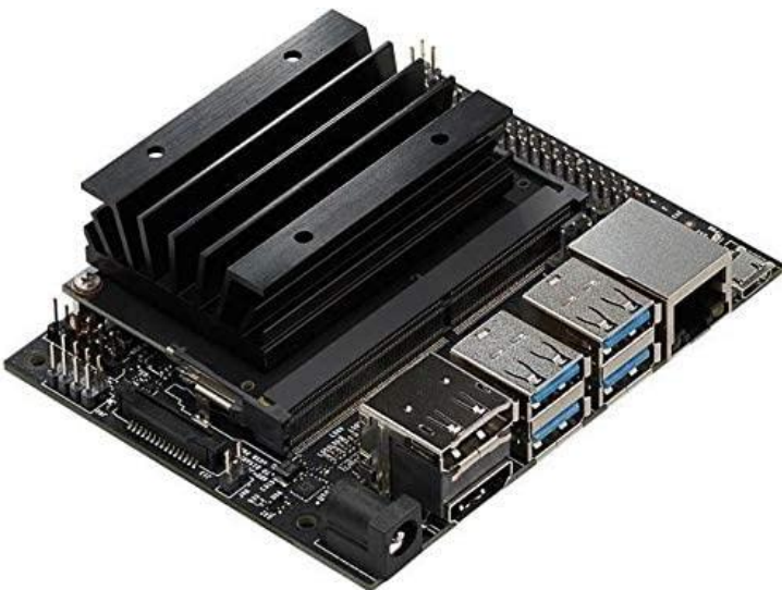
Figure 16. The Nvidia Jetson Nano computer used for AI/ML/CV tasks
