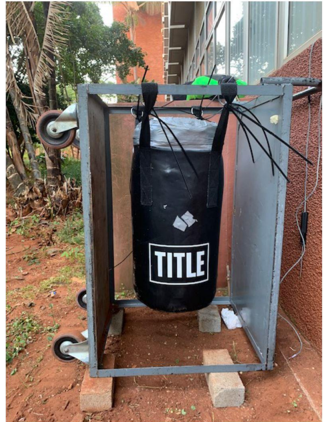
Fig. 2. The pre-heated Cooling Dummy vertically suspended and cooling outdoors in unforced convective conditions.
