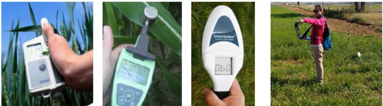
Figure 1: Several hand held optical sensors to measure crop nutritional status of the crop. The image on the right shows a more sophisticated field spectroradiometer used to compare the measurement of the commercial equipments.
