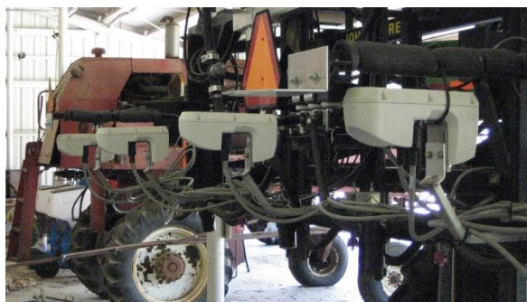
Figure 2. Sensors mounted on a variable fertilizer rate spreader.
