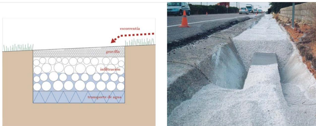
Figure 21. Pavement permeability (Madrid, 2009)
