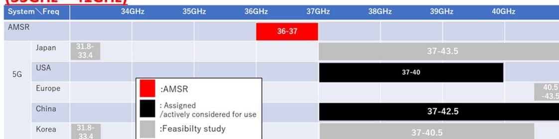
Figure 1: AMSR3 and 5G Allocated Frequencies. For 24.0-24.25 GHz, AMSR3 and 5G frequencies have a buffer band of 250 MHz. On the other hand, AMSR3 and 5G frequencies are adjacent to each other with no buffer band for 36-37 GHz. Its impact cannot be avoided by improving the out-of-band frequency characteristics while maintain the bandwidth.
