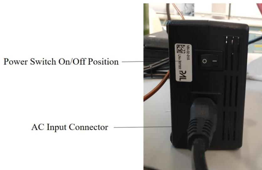
**Figure 4 Main power of the autosampler**
