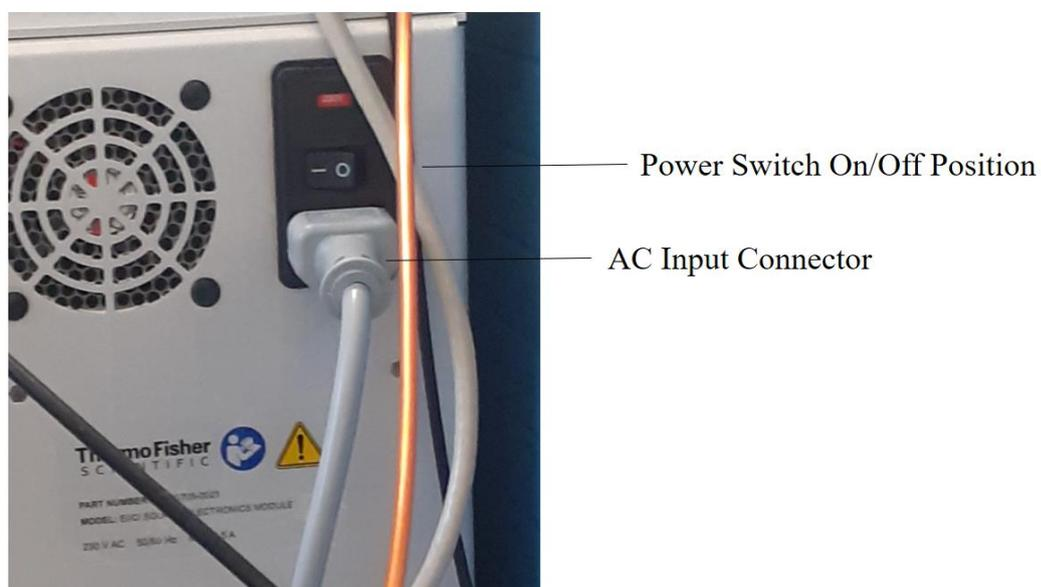
**Figure 3 Main power of GC transfer-line**
