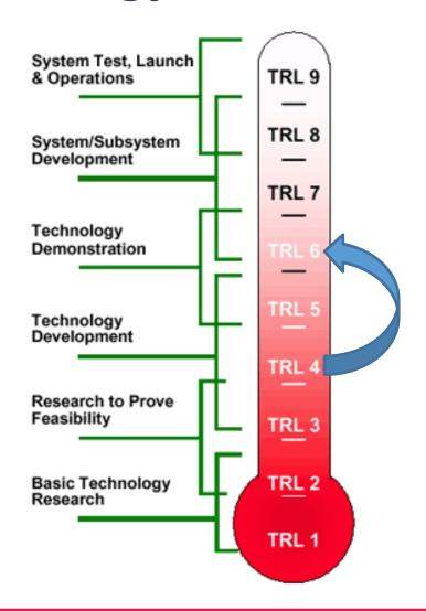
The three technologies will be advanced from the "lab-status" (TRL 4) to a technology demonstration level for inline/online process monitoring at pilot scale in the industrial environment (TRL 6) of the **NanoPAT** industrial partners.
