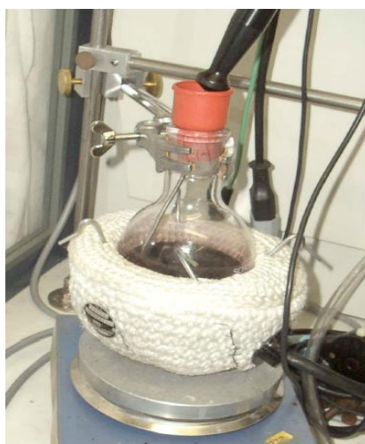
Figure 1.2.8. Au NPs are stirred after the addition of DDT while the temperature is controlled by a thermometer that is embedded in the reaction flask.
