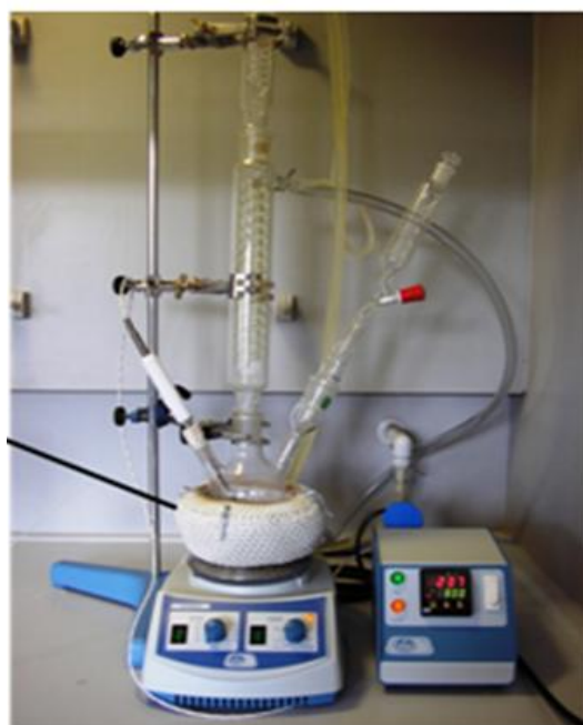
Figure I.7.1. Setup for the synthesis of CdSe/ZnS NPs. The photo shows a three-neck flask equipped with a heating mantle, a reflux condenser, an addition funnel, a thermometer connected to a temperature controller, and a nitrogen flow.
