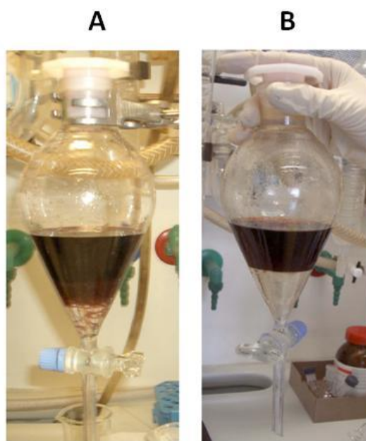
Figure I.2.5. Purification of TOAB-Au NPs. Upper toluene phase containing TOAB-Au NPs is washed with aqueous solutions (HCl, NaOH and Milli-Q water) in the lower phase to remove excess sodium borohydride and other residual chemicals. A) Photograph of the two phases immediately after shaking note that the two phases are not completely separated. B) Photograph of the two phases after they were allowed to separate forming a transparent aqueous phase at the bottom and a deep red organic phase at the top containing TOAB-Au NPs.
