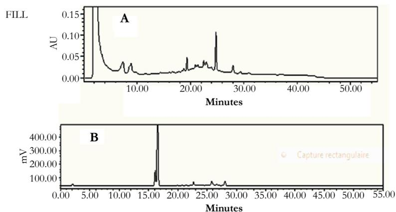
**Figure 7. Profile obtained by gas chromatography coupled to mass spectrometry. (A) Total ion chromatograms (TIC) of silylated investigated compound purified by HPLC-prep. (B) Typical EI mass spectra of TMS derivateives of oleanolic acid. (C) Typical EI mass spectra of TMS derivateives of ursolic acid.**
