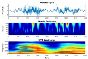
Figure 1: Comparison of different time-frequency representations. Top Row: Original speech signal. Second row: Wavelet Scalogram using a Mexican hat wavelet  $\psi(t)$ , which is also a particular case of the m-th order derivative of a Gaussian wavelet. Third row: Short Time Fourier Transform spectrogram.
