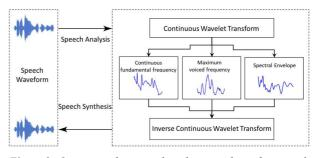
Figure 2: Overview of proposed analysis-synthesis framework using CWT-based approximation of speech features.
