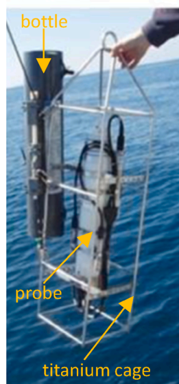
Fig. 1. (a) Image of the CTD and Go-Flo model bottle mounted in a titanium cage just before deployment in seawater. Reprinted from [9], Copyright 2020, with permission from Elsevier. (b) Schematic of the various platforms on which submersible sensors can be deployed. Image is reprinted from [16] with attribution 4.0 International (CC BY 4.0).
