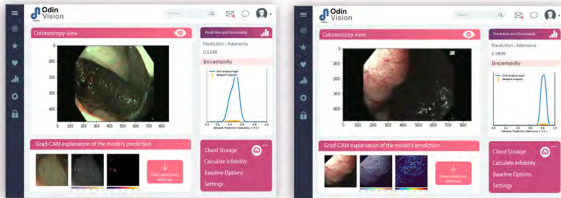
Figure 1: A proposed bespoke interactive dashboard: To identify potential failure modes and provide real-time rational of model predictions to clinicians using automated software. Two test cases are provided: (left) a false positive classification, (right) a true positive classification. Guided Gradcam provides the attributions (lower panel), and MC Dropout provides the uncertainty measure (right pannel). Dashboard was designed using Adobe illustrator and resources from Freepik.com
