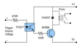
Fig. 4.Circuit diagram of relay module
