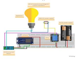
Fig. 8. Circuit diagram of custom IOT device
