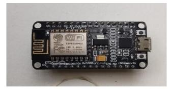
Fig. 3. NODEMCU AMICA V1.0 Development Board
