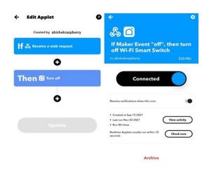
Fig. 10. Integration of webhooks and device's mobile application in IFTTT
