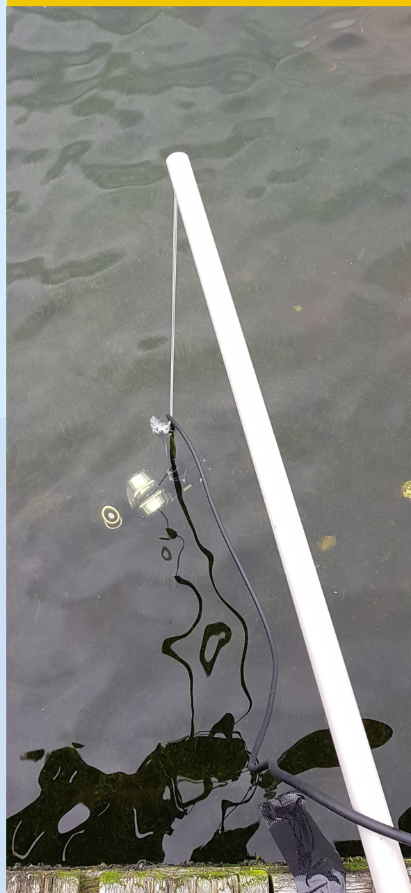
Measurements with different modules of KduPRO and Li-COR Li-192 reference sensor
