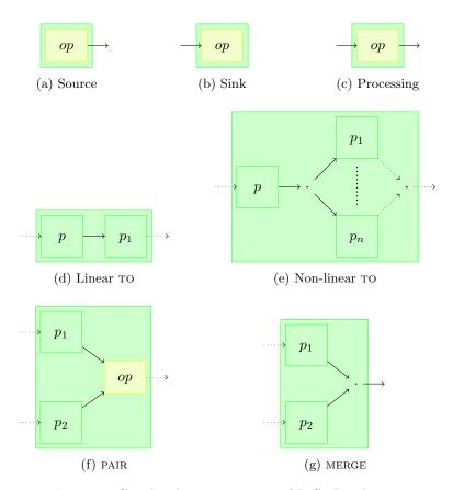
Figure 1: Graphical representation of PiCo Pipelines
