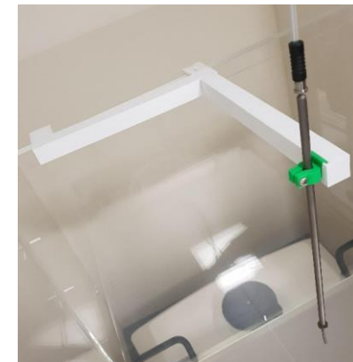
Above: Brachy holder for water tank, and measurements performed using it
