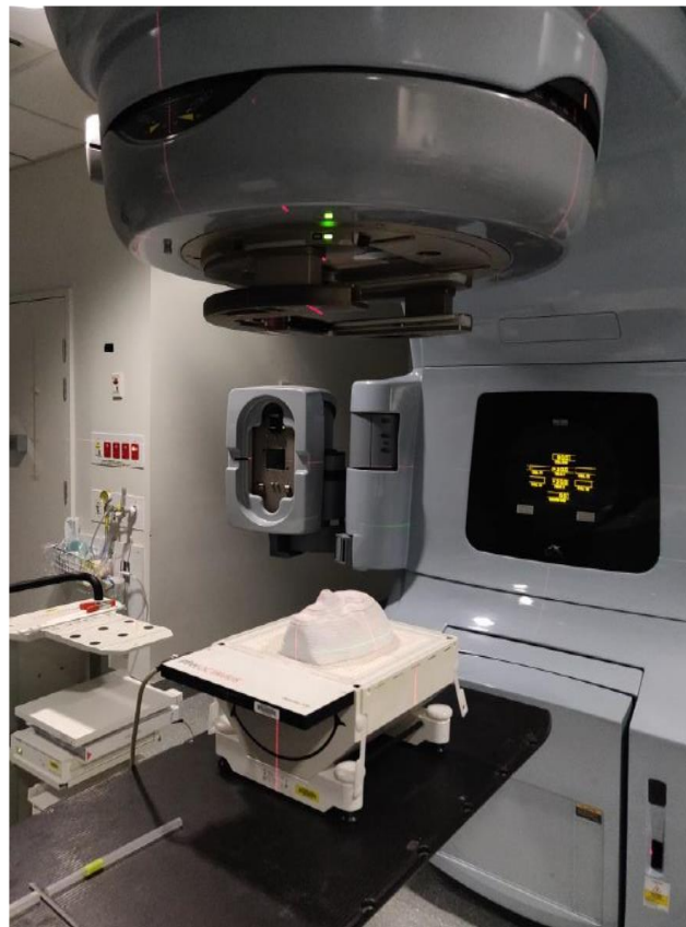
Left: coronally sliced head phantom and planar dose measurements.
