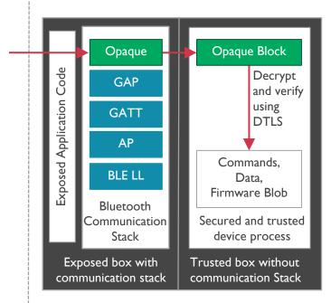
IoT Device owned by user. Initial identity provisioned by System Integrator Messages delivered agnostic of communication stack
