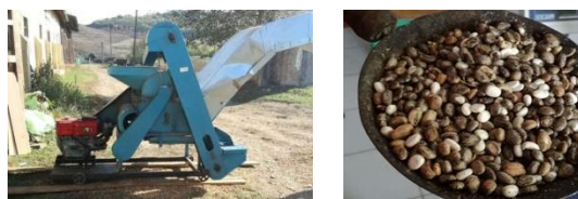
Figure 1: Dehusking machine (left) and the seeds obtained (right) after the fine regulations.
