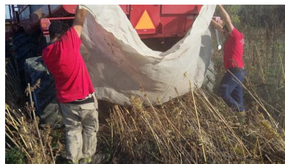
Figure 3: Evaluation of seed losses due to the inefficient setting of the threshing elements
