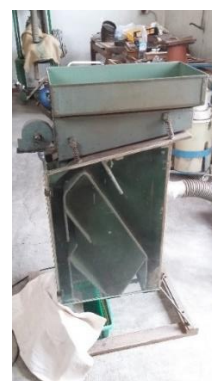
Figure 4: "Seed blowing machine" to separate seeds from soil and from empty seeds
