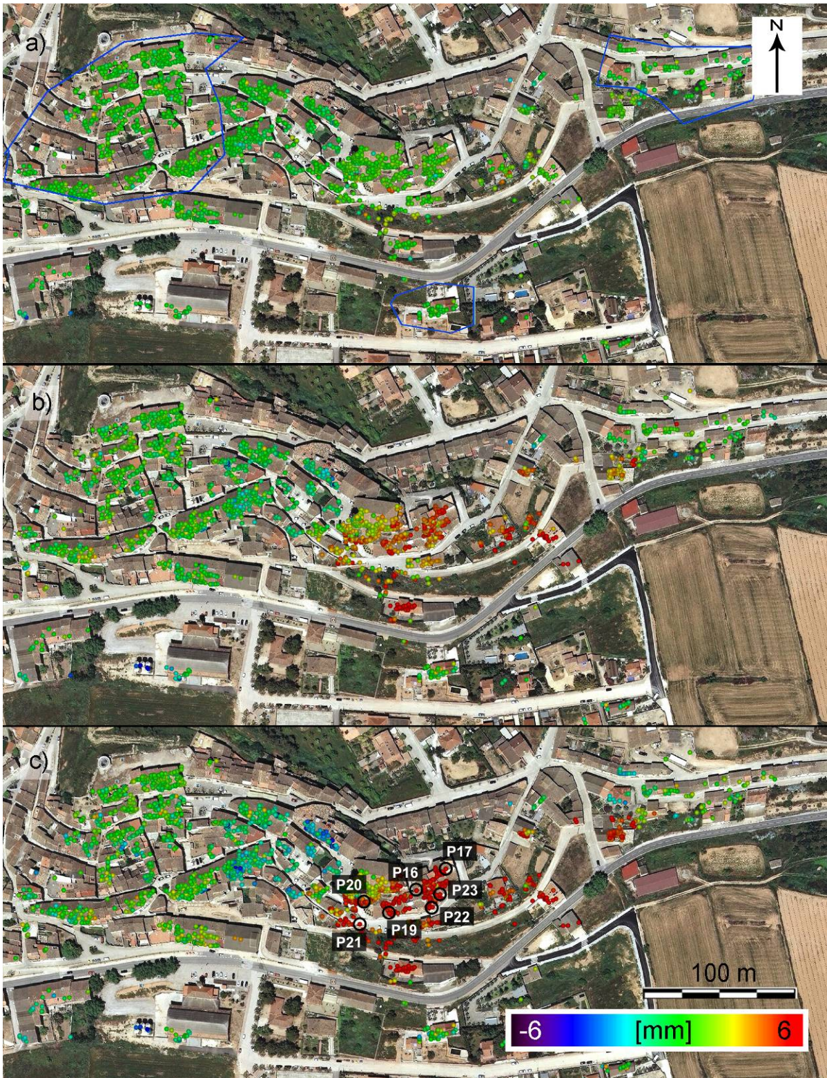
Figure 4. Displacement maps of Barberà de la Conca between the first campaign (14/11/2011) and the campaigns of 19/12/2011 (a), 08/05/2012 (b) and 20/03/2013 (c). The blue polygons on the top indicate the stable areas.
