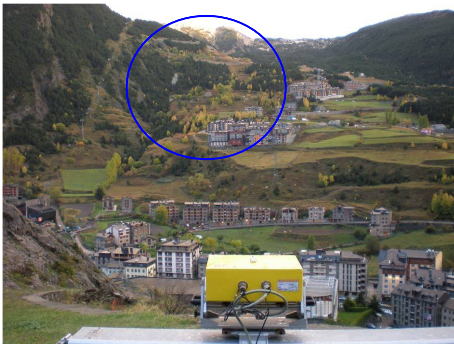
Figure 6. Photograph of the measured scene in the second case study, taken from the radar viewpoint. The blue circle highlights the main area of interest, which is located between 1000 and 1600 m from the radar.
