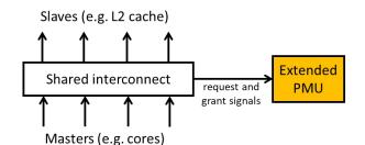
Figure 3. Extended PMU for a shared interconnect
