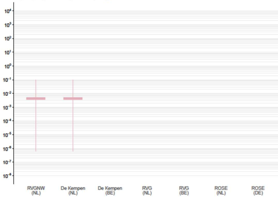
Hydraulic conductivity [m/d] of MSk2 by model area Expert (box) and data (whiskers) ranges
