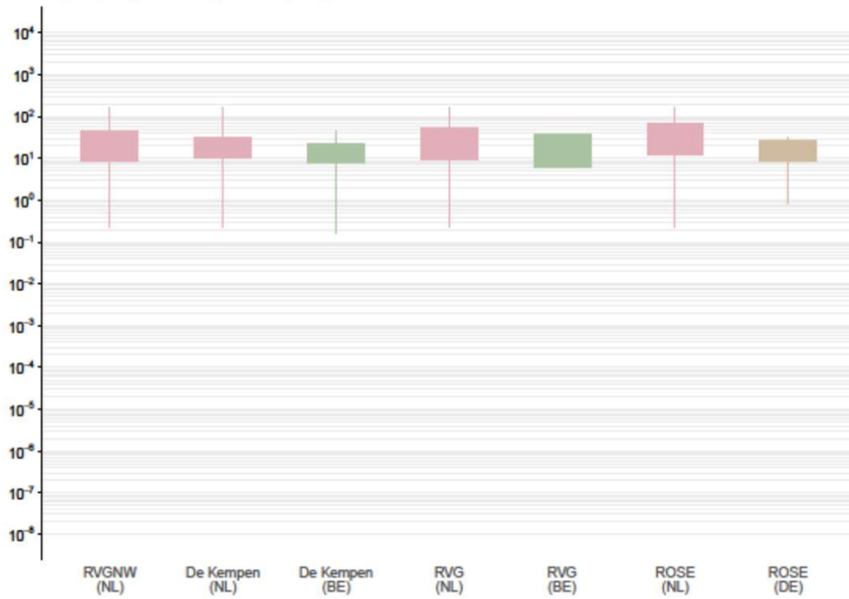
Hydraulic conductivity [m/d] of Klz3 by model area Expert (box) and data (whiskers) ranges
