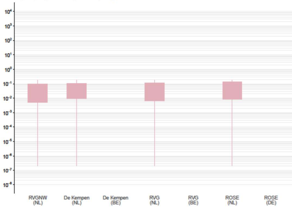
Hydraulic conductivity [m/d] of SYk1 by model area Expert (box) and data (whiskers) ranges
