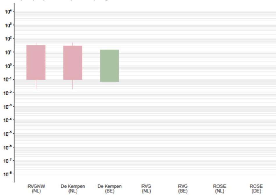
Hydraulic conductivity [m/d] of OOz2 by model area Expert (box) and data (whiskers) ranges
