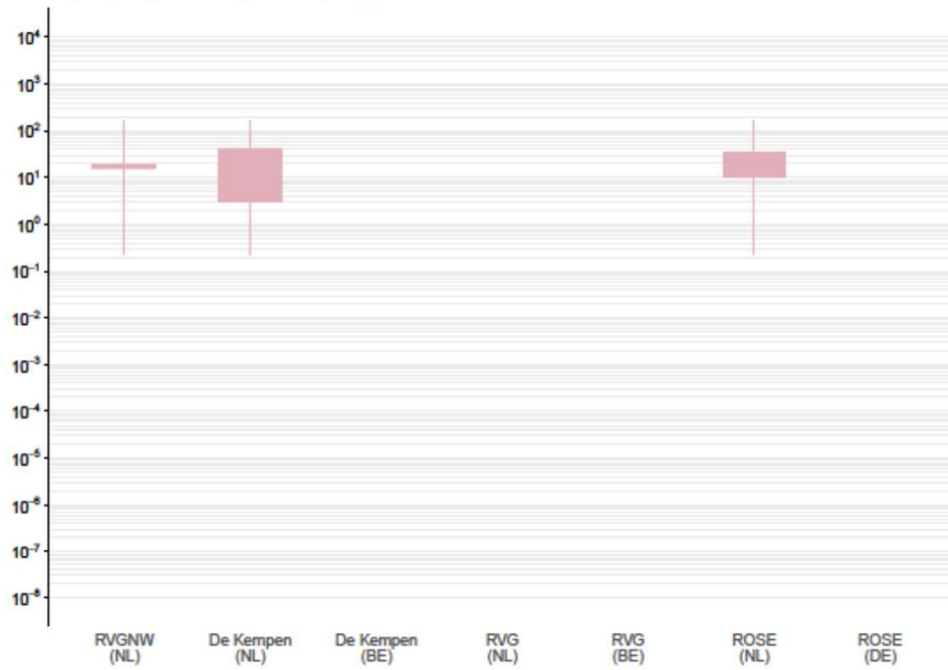
Hydraulic conductivity [m/d] of Klz1 by model area Expert (box) and data (whiskers) ranges
