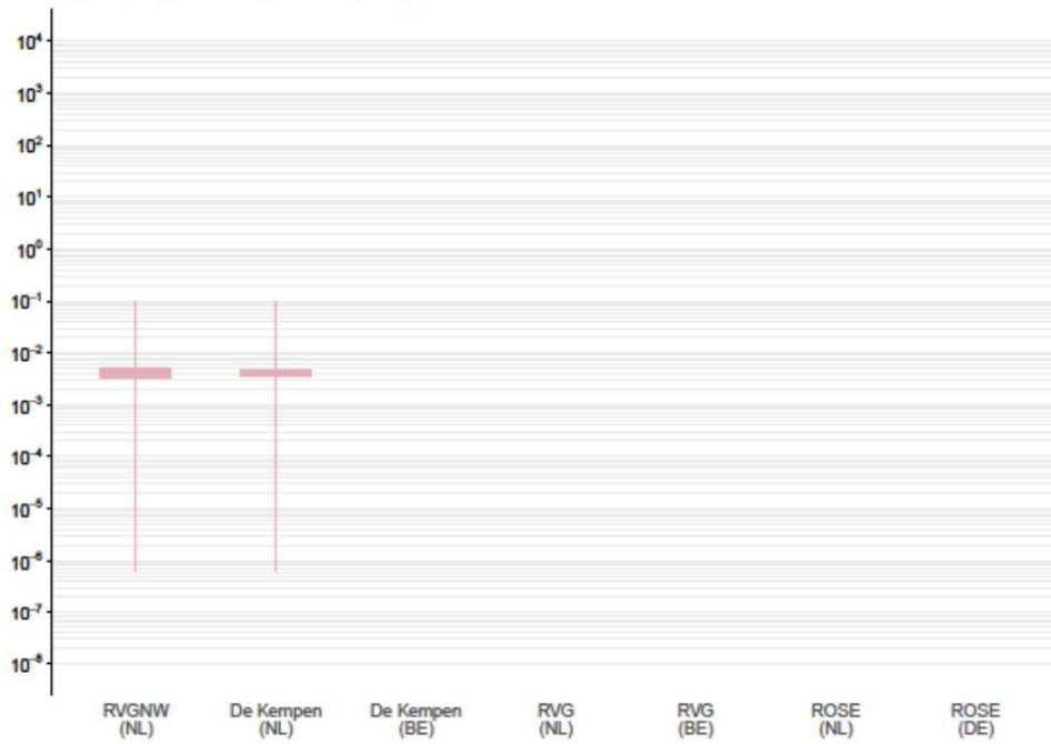
Hydraulic conductivity [m/d] of MSk1 by model area Expert (box) and data (whiskers) ranges
