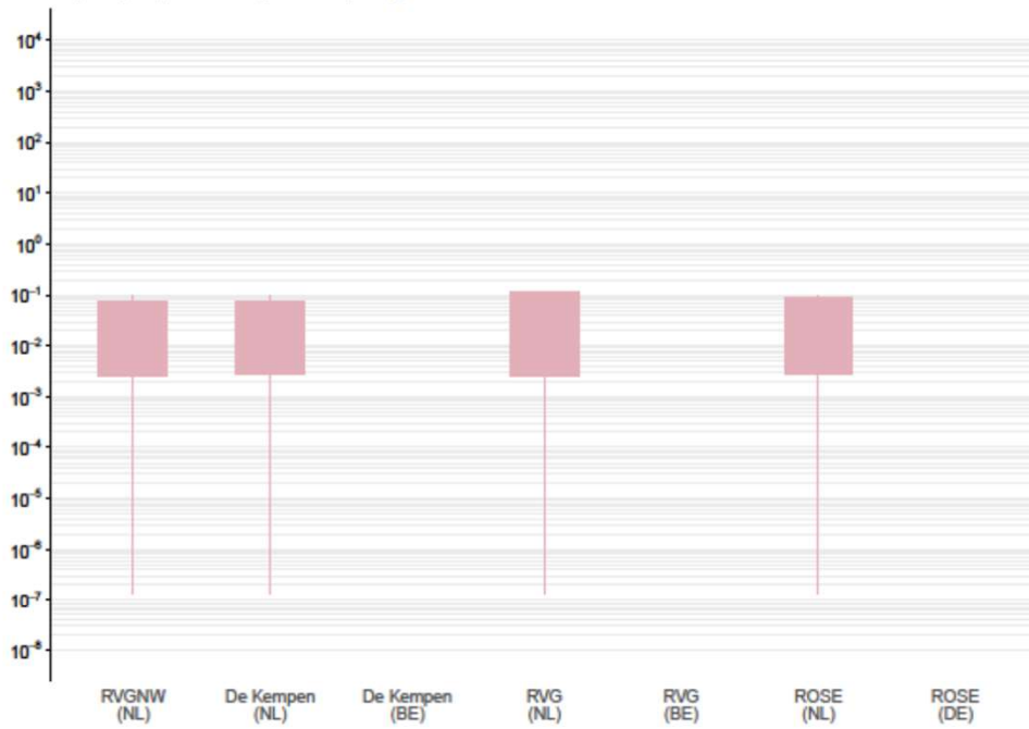
Hydraulic conductivity [m/d] of WAK2 by model area Expert (box) and data (whiskers) ranges
