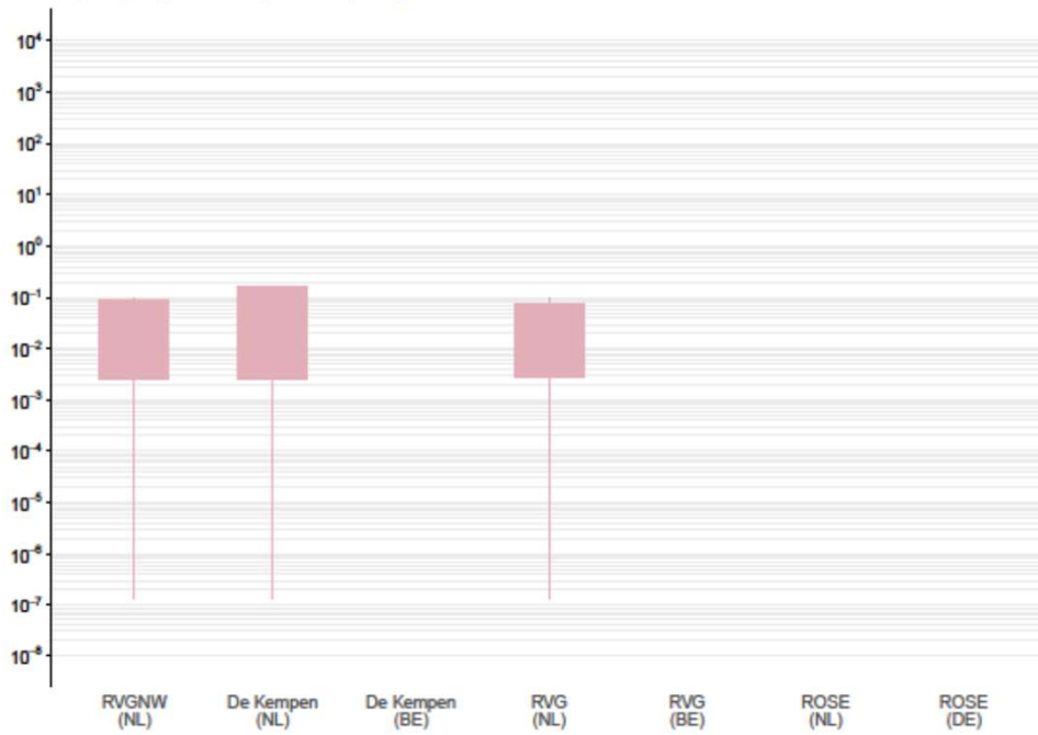
Hydraulic conductivity [m/d] of WAK3 by model area Expert (box) and data (whiskers) ranges
