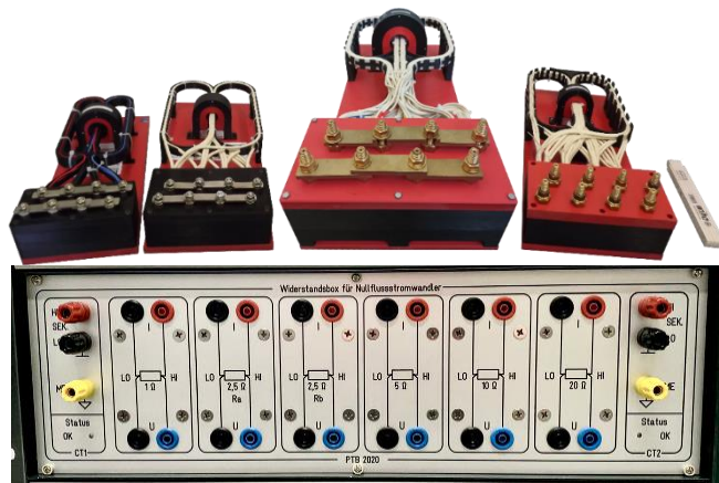
Fig. 7. Photo of the accomplished wideband current-to-voltage transformer set for currents up to 2 kA. The symmetrical current transformers (above) and the front panel of the associated precise measuring resistor box (below)
