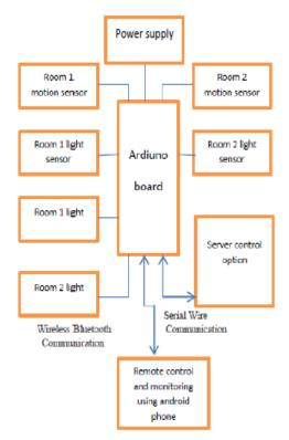
Fig 4: Block diagram of Intelligent Lighting System
