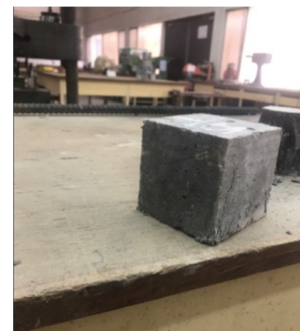
Fig. 2. The typical failure behavior of concrete specimens with 2% PP fibers under compression.
