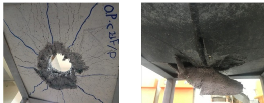
Fig. 8. Typical failure behavior of concrete specimens including 2% PP fibers and polymer grids under impact.
