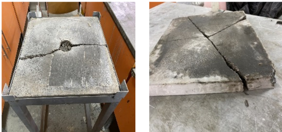
Fig. 4. Typical failure behavior of unreinforced concrete slabs.
