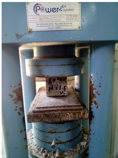
Fig. 2. Compressive strength test.
