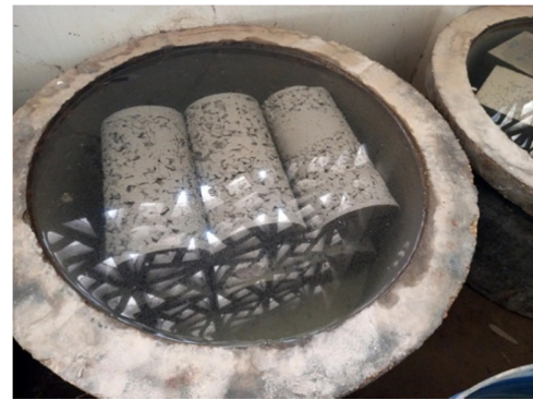
Fig. 5. Curing of specimens.
