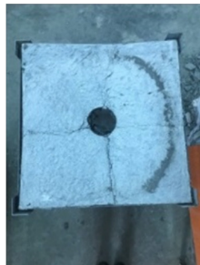
Fig. 9. Typical failure behavior of concrete specimens including 2% PP fibers and steel grids under impact.
