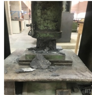
Fig. 1. The typical failure behavior of reference concrete specimens.
