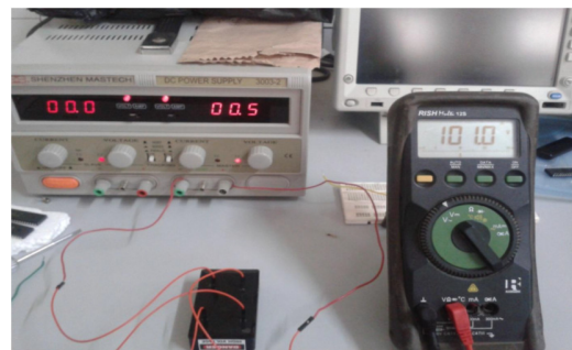
Fig. 4. Boosted voltage displayed in voltmeter.
