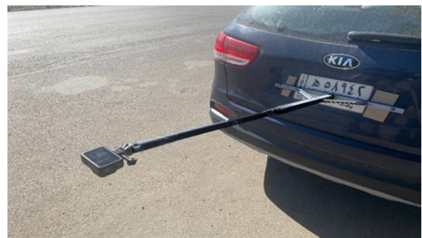
Fig. 2. The angle between the camera and the surface of the pavement.
