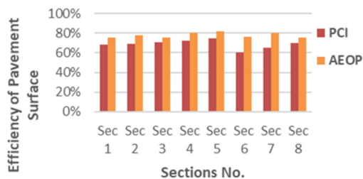
Fig. 5. Percentage differences between PCI and AEOP surveying.
