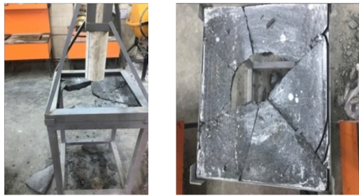
Fig. 7. Typical failure behavior of reference concrete specimens under impact.
