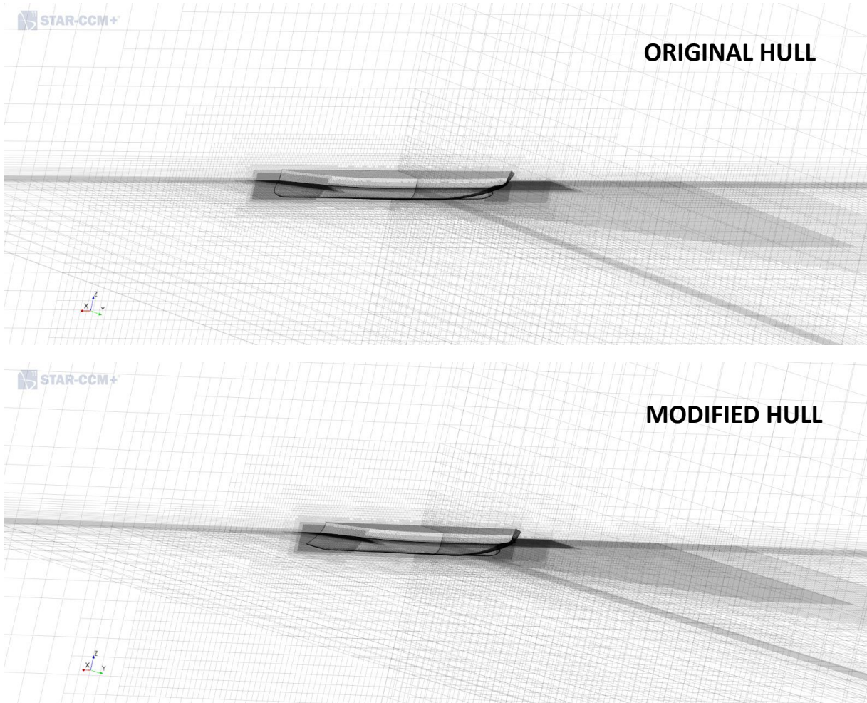
Figure 11: 3D mesh, 4 million elements, RANS solver
