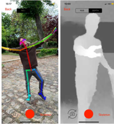
Fig. 3: Example of the smartphone application using the skeleton visualization module and the rear camera (left image) and the recording module of the application enabling the depth visualization with the true depth camera (right image)
