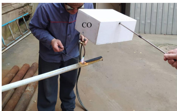
Fig. 1. The process of studying the concentration of aerosols, which are formed during gas welding using the signaling device-analyzer DOZOR-S-M
