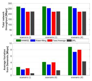
**Fig. 3.** Comparison amongst methods: DRL performance against *Waterfilling*, *WMMSE* and *Fixed Average* methods for the different validations scenarios in terms of total network throughput (up) and *AVD* (down) across 1000 network realizations.
