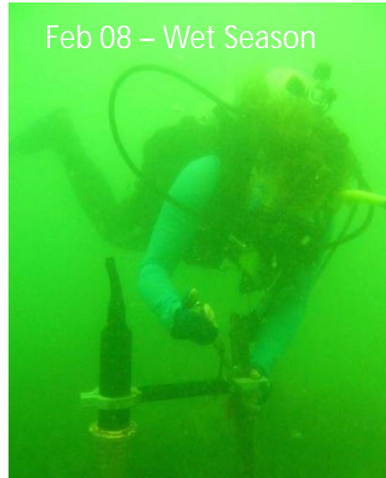
WET Labs Eco FLNTU (Fluorometer and Turbidity Sensor) at Barren Island
