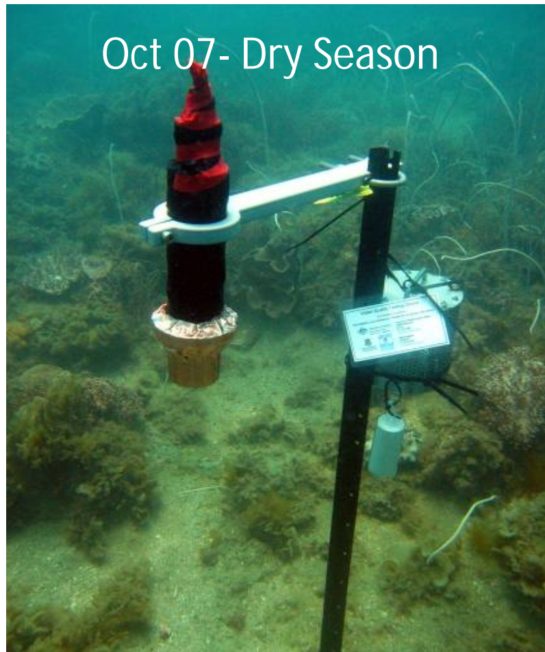
WET Labs Eco FLNTU (Fluorometer and Turbidity Sensor) at Barren Island
