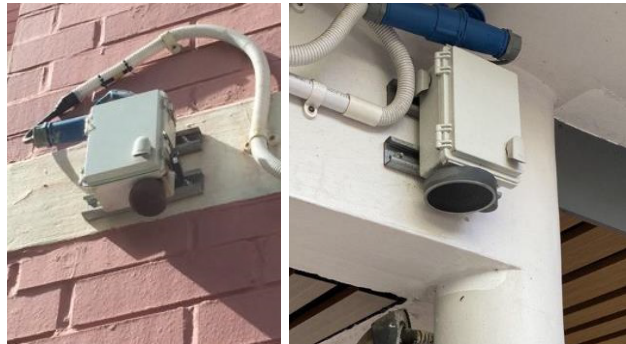
Fig. 1. Sensor units used to make recordings for the SINGA:PURA dataset. Left : A unit with a single-channel SPH0645 microphone. Right : A unit with a seven-channel UMA-8 v2 microphone array.
