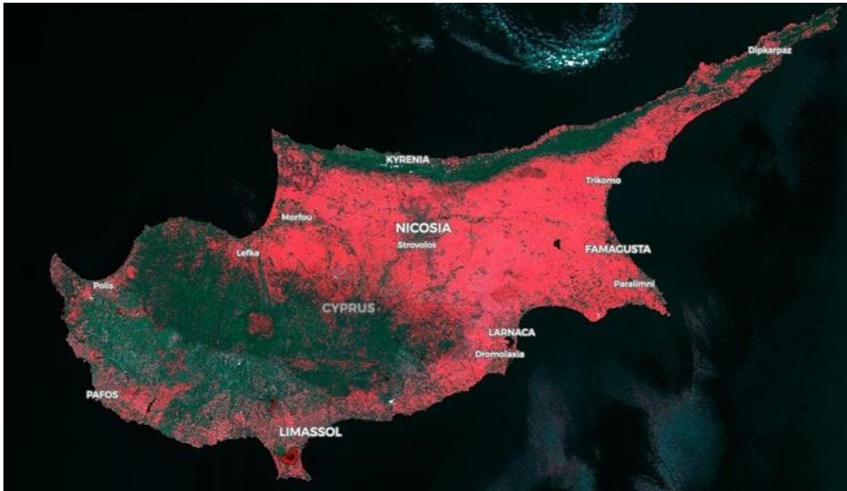
Figure 15: An overview of the bare-soil classifier over Cyprus, taken on 2020-05-13. The red color marks the detected bare soil (credit: European Union, contains modified Copernicus Sentinel data 2020, processed with EO browser).
