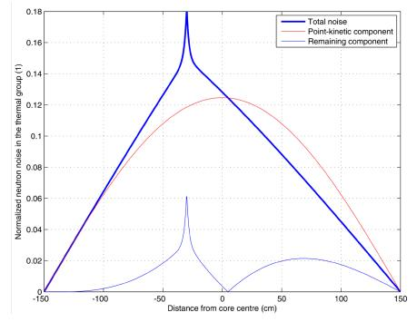
Illustration of the difference between the point-kinetic component and the total induced neutron noise in the frequency domain at 1 Hz, for a perturbation located at -30 cm from the centre of a nuclear core of size 300 cm.
