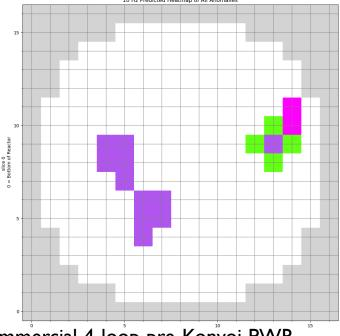
Example of machine learning-based unfolding at 10 Hz in a commercial 4-loop pre-Konvoi PWR Figure from Durrant, A., Leontidis, G., Kollias, S., Torres, L.A., Montalvo, C., Mylonakis, A., Demazière, C., Vinai, P. (2021), Detection and localisation of multiple in-core perturbations with neutron noise-based self-supervised domain adaptation. Proc. Int. Conf. Mathematics and Computational Methods Applied to Nuclear Science and Engineering (M&C2021), Raleigh, NC, USA, October 3-7, 2021
