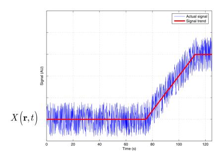
Conceptual illustration of the possible timedependence of a measured signal from a dynamical system
