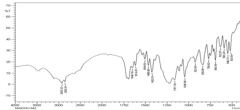
Figure 4: FT-IR of spectrum of physical mixture of drug and fumaric acid.
