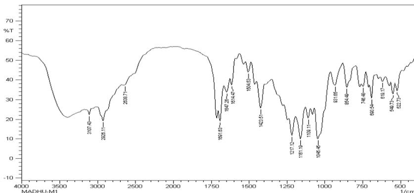
Figure 3: FT-IR of spectrum of physical mixture of drug and tartaric acid.
