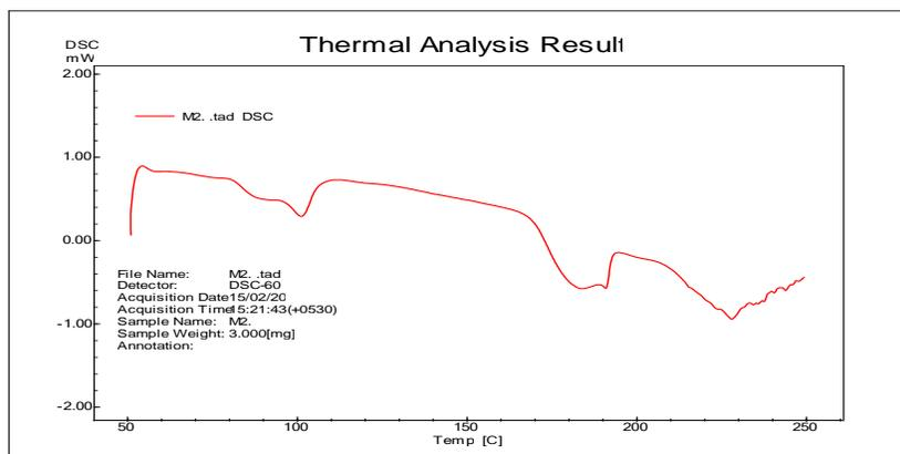
**Figure 8: DSC spectrum of physical mixture of drug and fumaric acid.**
