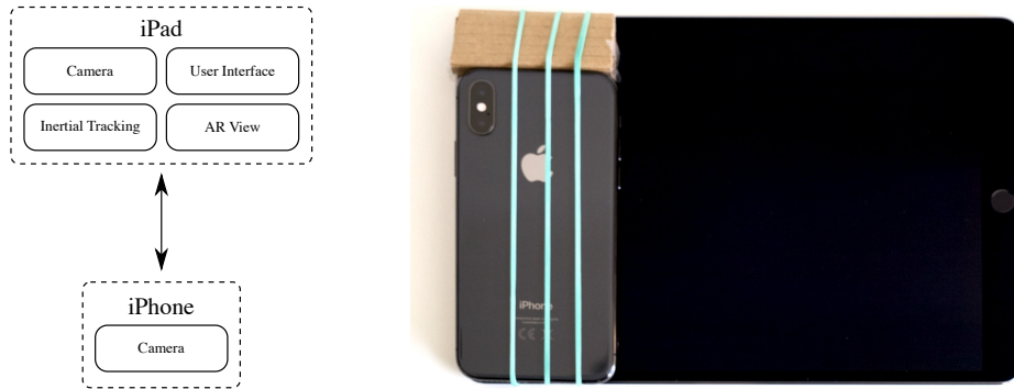
Fig. 1: Left: The tracking system consists of two components: an iPad (receives the data from its rear camera, its IMU, and the user, and displays the AR content), and an iPhone (receives the data from its rear camera). Right: The iPhone being placed on the iPad device with its rear camera directed behind the user, and together, the devices work as one stable unit.
