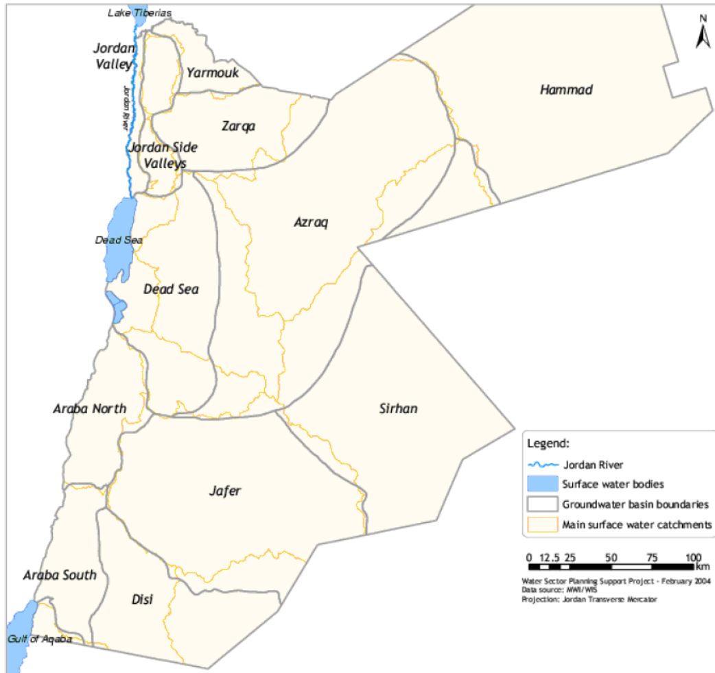
Fig. 2 shows the spatial distribution of the surface water catchments and their relative position to the groundwater basins. The high water demand is met by over-abstracting the renewable groundwater aquifers. (NWMP, 2003).
