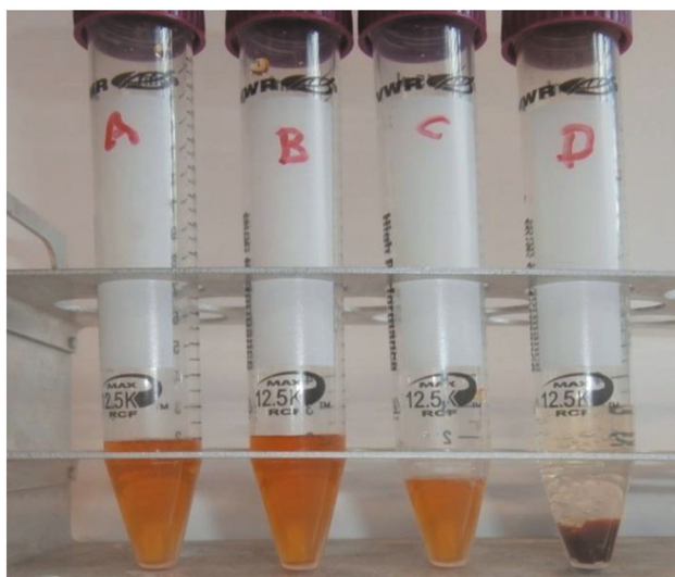
Fig. 9. Optical images of the aqueous solutions of \text{Fe}_x\text{O}_y NPs after 3-day equilibration. The samples were prepared at different nucleation temperatures T_N : 22 (A), 37 (B), 41 (C), and 45^\circ\text{C} (D).
