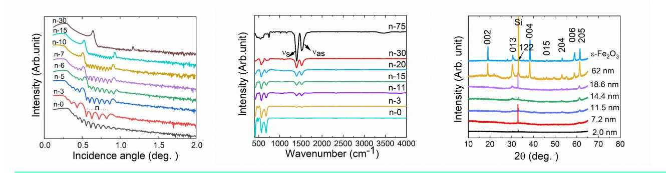
Grain size increases with decrease of individual iron oxide thickness
