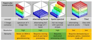
Fig. 10. Different ways to sample hyperspectral data [VITO].
