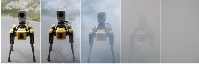
Fig. 8. The view of Spot from inside the tent at approximately 2 m distance. With increasing fog, the visibility decreases up to a point where spot is not observable any more.
