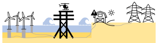
Fig. 1: Electricity transmission from turbines to offshore substation to onshore substation and finally to the power grid.
