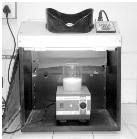
Fig. 1. Experimental setup for degradation of petroleum industry wastewater.
