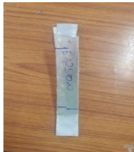
Figure:10 Delamination of GLARE. at 45 degree after tension test. Each metal layer is 0.6 mm thick
