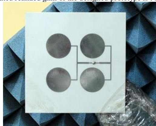
Fig. 8 Photograph of the fabricated antenna array.
