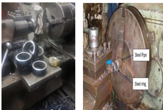
Fig. 6 Cutting the steel rings
