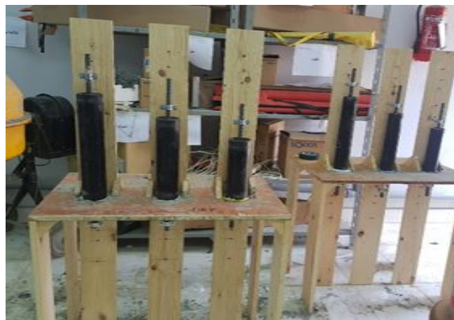
Fig. 7 install the bars to be spliced
