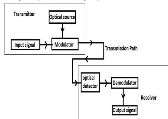
Figure 1.1: Block diagram of Optical fiber communication system [10]
