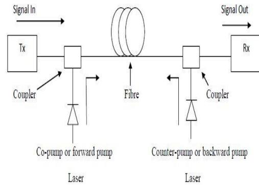
Figure 1.10: basic block diagram of Raman Amplifier
