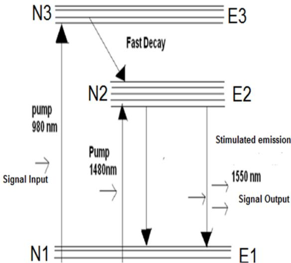
Figure 1.9: Three level energy diagram of  $\text{Er}^{3+}$  ions [15]
