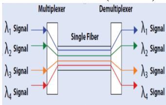
**Figure 1.4: Block diagram of Wavelength division multiplexing [8]**
