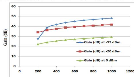
Fig 4.2: Variation of Gain with different pump power of proposed C-band EDFA with respect to three different input powers.
