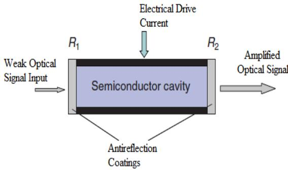
Figure 1.7: Basic diagram of Semiconductor Optical Amplifier (SOA) [14]
