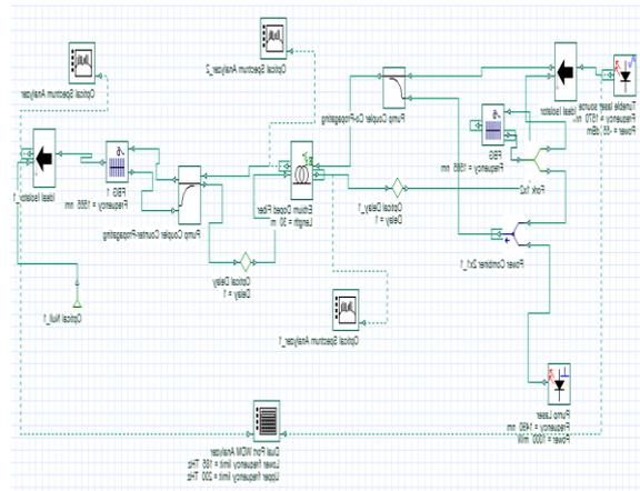
**Figure 3.1: Simulation setup of proposed EDFA with ASE reinjection**
