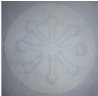
Figure 3: Fabricated μPAD with the PVA barrier.
