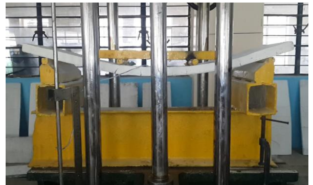
Fig.7 Flexural Strength Test in progress
