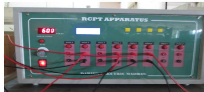
Fig. 2. Rapid Chloride Penetration test in progress
