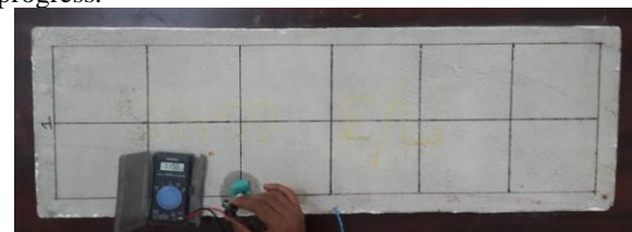
Fig.3 Half-Cell Potential test in progress
