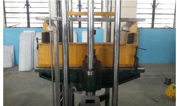
Fig.6 Flexural Strength Test Set up
